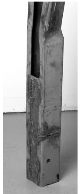
Damaged column repaired by electrode welding (Photo: Maurice Vézinnet)
