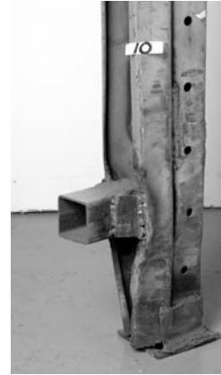
Damaged double column: Substandard weld, worn and deformed column due to friction with the lift truck outriggers (Photo: Maurice Vézinnet)
