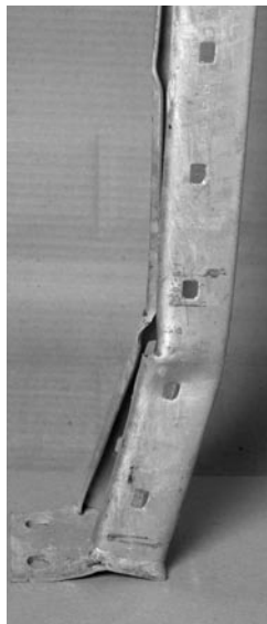
Same damaged column (Side view) Photo: Maurice Vézinnet
