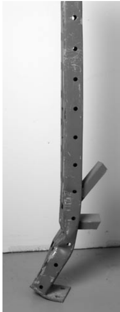
Same damaged column (Side view) (Photo: Maurice Vézinnet)
