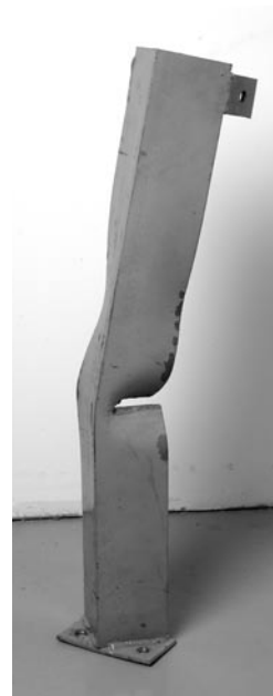
Damaged column guard (Photo: Maurice Vézinnet)
