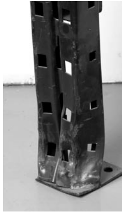
Damaged column: The weld near the base plate gave way (Photo: Maurice Vézinnet)
