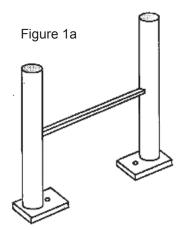
Bearing plates are placed under each post
