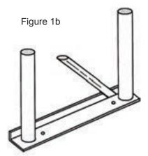
A continuous bearing plate joining the two posts
