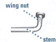
Figure 32b. Recommended as a lock pin design
